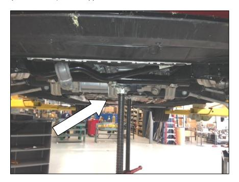
18. Remove the 4 bolts for the front of the subframe.
