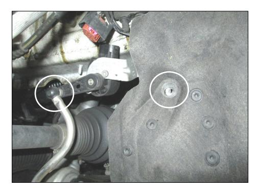
15. Remove the two bolts on both sides of the subframe going to the front bumper, then remove the wire holder from the frame.
