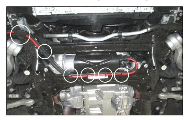
9. Disconnect the two plugs of the rack and move it out of the way.
