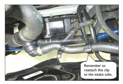
30. Rotate the swaybar and verify that there is 1/2" of clearance with the hose. Adjust the length of the hose mount if necessary.
