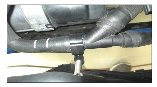
Take the smaller I" clamp and secure it to the upper hose as shown.
