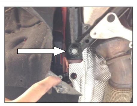
17. Use a pole or floor jack to support the front of the subframe.
