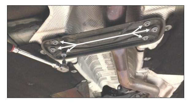
3. Remove the 4 nuts from both lower control arm covers. Remove covers and set aside.
