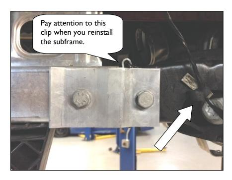
16. Loosen the two subframe rear bolts. Only loosen these bolts two or three turns at the most!
