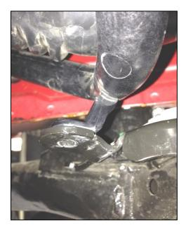
8. Remove the 6 clips that secure the wiring harness for the steering rack.
