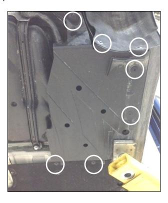
9. Use pole or floor jack to support the front of the differential housing as shown.
