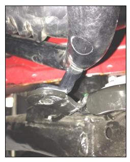
8. Remove the 4 clips that secure the wiring harness for the steering rack.
