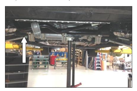
• Move the bar further to the left and rotate as needed to remove the bar from the bottom.
