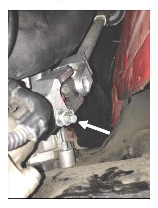
12. Remove the 3 bolts from both sides of the motor mount.
