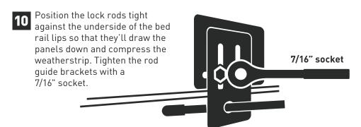
To get the weatherstrip compression necessary for its adhesive to cure and the cover to keep out the weather, have a second person press down on the cover while you're adjusting the lock rods.
