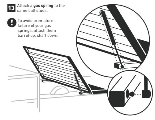
14 Attach the three remaining gas springs (barrel up, shaft down).
