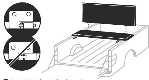
To avoid hinge damage, do not close the panel until the hinges are fully mated: With the panel tilted more than 90° from its closed position, slide it onto its hinges until the hinge barrels are aligned with the leaves and the locking tabs interlock.
