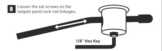
Adjust the length of the lock rods and retighten the set screws so that:
