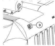
Install hand wand clip using 1-10/24 truss head screw as shown (B).
