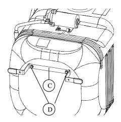
Install hose tender bracket (C) using two 5/16 x 5/8 in. flange bolts (D).
