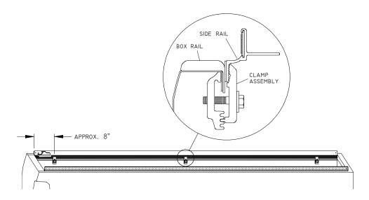
**B)** Adjust side rails: For optimum latching performance and cover fit, side rails must be level. To adjust rails, loosen screws and reposition male clamps higher or lower. Tighten all clamps.
