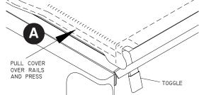
**B)** To release cover, pull back on toggle. Leaving VELCRO® brand hook and loop attached, roll cover toward cab to open.
