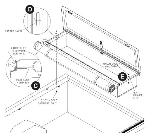
**E)** Secure toolbox to side rails with 5/16" x 3/4" carriage bolts, flat washers, and lock nuts.
