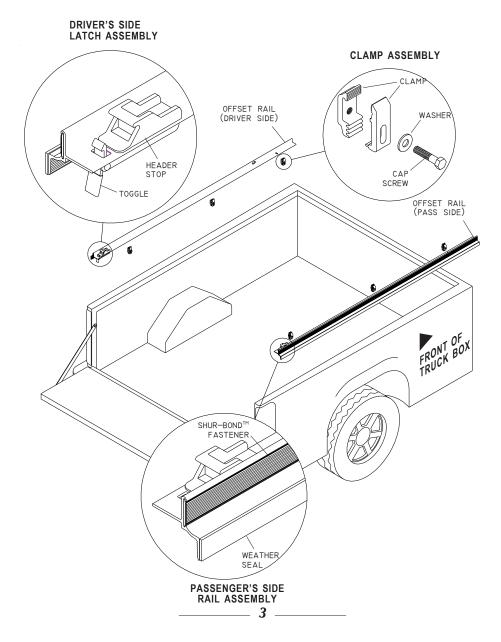
**A)** Install side rails: Place side rails against front of truck box, flush with box rail and level with each other. Starting at tailgate, evenly space three clamps along each side rail, leaving about 8" free on each end.
