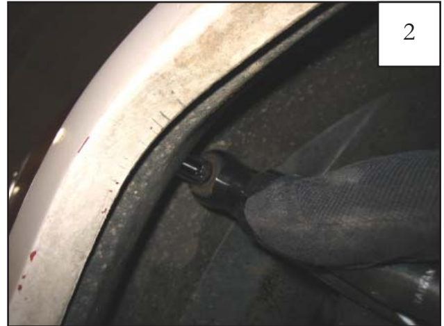
2 Using a 10mm socket, remove the factory fastener located inside the top front of the fender well.
