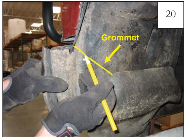
At the front of the splash shield, draw a line from the area cut in Step 19 down to the plastic grommet, taking care not to cut through the grommet. Trim on this line.
