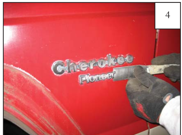
4 Apply adhesive remover to the Cherokee emblem for ease of removal. Using a putty knife, carefully remove the Cherokee emblem, taking caution not to scratch the paint.
