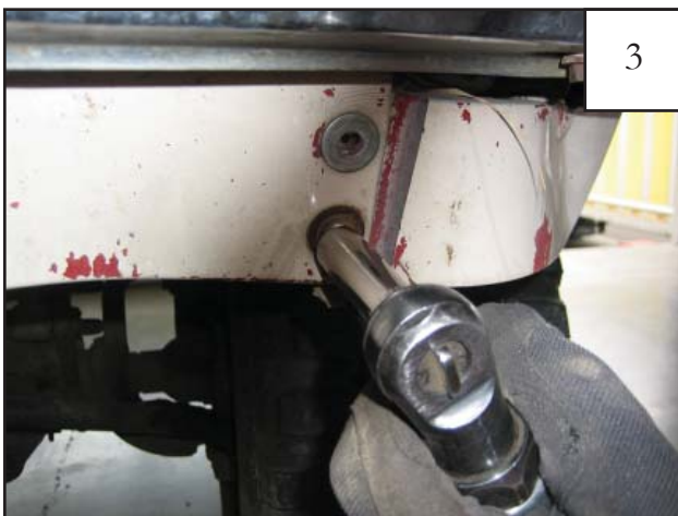
3 Using a 10mm socket, remove two factory fasteners underneath bumper on either side. Remove fascia piece.
