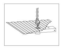
pecially if the truck bed floor has been distorted downward from heavy use. If you use an overhead-lifting device, it should be disconnected before squaring the center section across the frame, installing the side-plates and torquing fasteners.
