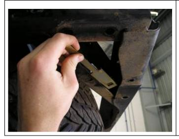
28. Fit M12 x 1.75 cage nut into rear cross member nut plate and fit to both sides of rear cross member.
