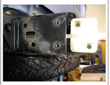
21. Whilst working on the LHS, fit M12 x 1.75 caged nuts into side plates, and fit plate as to press wing brace nut plate arm against the inside of the chassis rail to stop any rattling when the rear bar is fitted to vehicle.
