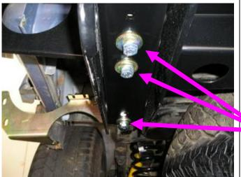
32. Fit 3 x M12 x 40mm x 1.25 (fine thread) bolts, spring washers and large gold colored flat washers to underside of chassis rails to LHS of vehicle (Finger tighten only.)
