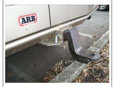
60. Fit gooseneck with pull pin and spring clip as shown.
