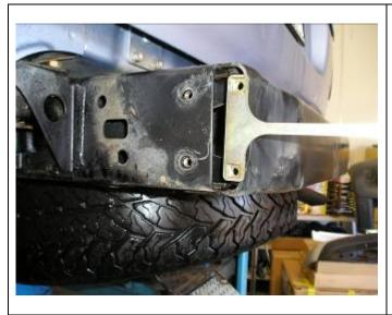
19. Fit 8mm cage nuts to wing brace nut plate and insert into LHS of vehicle and align with rear holes in side of chassis
