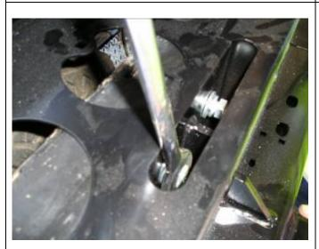
31. Fit two **M12** x **40** x **1.25** bolts, spring washers and flat washers as shown into centre mounting bracket.
