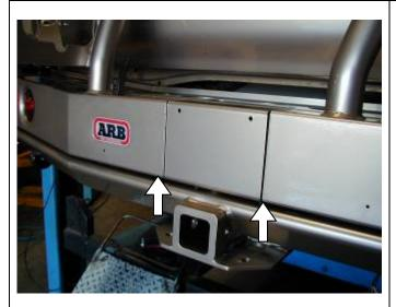
43. Align faces of centre cover panel with wheel carrier, jerry can carrier or cover panel and tighten securely.
