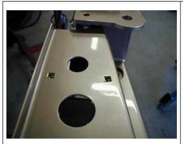
9. Fit M6 cage nuts (9 total) in square holes in top of bar as shown.
