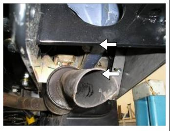
48. Using **M8 x 20 bolts**, flat washers and flange nuts secure end surrounds to braces finger tight. (RHS shown.)
