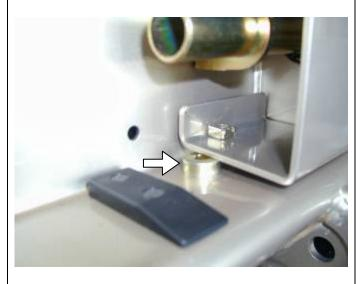
41. Place 8mm spacer between underside of centre cover panel and rear bar.
