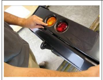
18. If a wheel carrier or jerry can carrier is not to be fitted a cover panel must be fitted.
