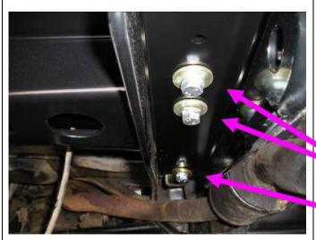
To the RHS of the vehicle, fit 2 x M12 x 1.75 x 50 (coarse thread) bolts, spring washer and flat large gold coloured washer to the most forward hole. To the rear hole, fit 1 x M12 x 1.25 x50 bolt, spring washer and flat large gold coloured washer
