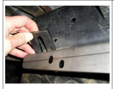
35. The single cut out packers to the front of the bar. (As viewed from front of vehicle) When these packers are fitted, tighten all bolts firmly.
