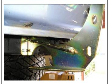
20. With the help of a friend to hold the previously fitted nut plate in the correct position, fit the LHS end surround brace to the side of the chassis rail using M8 x 35mm bolts, spring washer and flat washer., finger tighten only.
