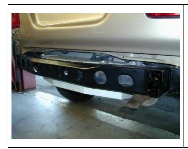
13. To fit Rear Bar to vehicle, remove bumper bar, mud flap and tow bar (if fitted) from vehicle.
