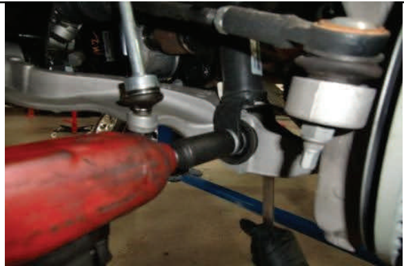
Remove lower strut mounting nut.
