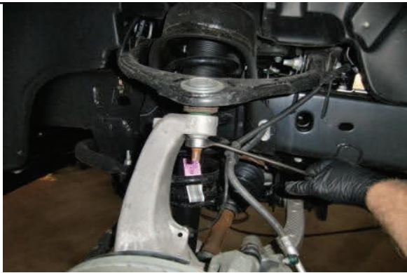
Loosen upper ball joint nut. Leave attached.
