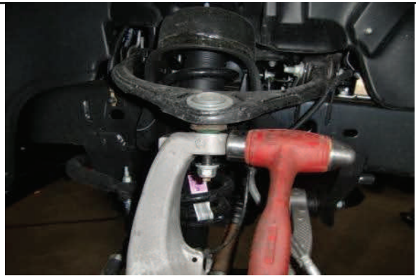
Carefully strike spindle to break upper ball joint loose.
