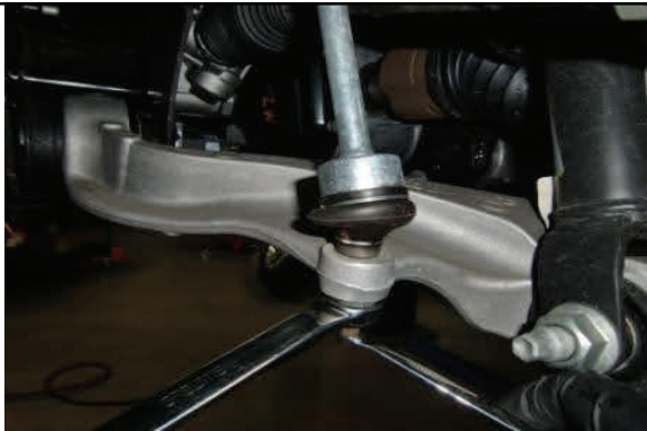
Loosen and remove lower sway bar nut.
