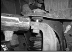
5. Working on the driver side, remove the stock lower sway bar end link hardware. Set the stock hardware aside. Remove the stock end link from the stock lower control arm. Repeat procedure on the passenger side.
