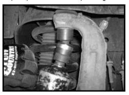
4. Working the driver side, carefully break the stock taper on the stock upper control arm and the stock knuckle. Special Before installation begins, measure from the center of note: Carefully hitting the stock knuckle with a hammer damage the stock upper ball joint boot. Do not remove the stock nut at this point. Repeat the procedure on the passenger side.
