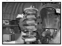
11. Locate the new strut spacers and the stock hardware. Working on the driver side strut, install the new spacer on top of the stock strut and secure using the stock hardware. Make sure to use thread locker or loctite and torque to **48 ft lbs**. Repeat procedure on the passenger side strut.
