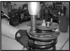
12. Locate (6) 3/8" nylon lock nuts and (6) 5/16" USS flat washers from hardware bag D2P-NB. Working on the driver side, install the modified passenger side strut into the stock upper driver side location and secure using the new 3/8" hardware. **Do not tighten at this point.** Repeat procedure holding the stock upper control arm to the stock knuckle and on the passenger side with the driver side strut.
