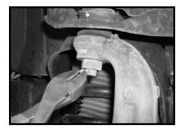
stock nut connecting the stock upper ball joint to the stock knuckle. Repeat procedure on the passenger side.
