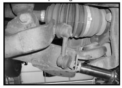
Locate the stock upper control arm mounting hardware. Working on the driver side, attach the stock upper control upper control arm down so that it can be attached to the stock knuckle. Repeat procedure on the passenger side.
