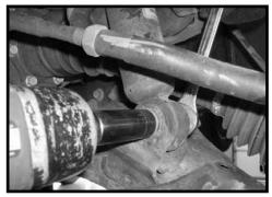
14. Locate the stock lower sway bar end link hardware. Congratulations, installation complete! Working on the driver side, install the stock end link into the stock location and secure using the stock hardware. Make Special note: After the completion of the installation, sure to use thread locker or loctite and torque to 42 ft lbs. Repeat procedure on the passenger side.
