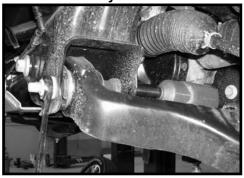
With both strut assemblies out of the vehicle it is time to install the new leveling spacers. Install these directly on top of the stock strut cap and secure them using the stock nuts. 15. Working on the driver side re-install the tie rod ends back Torque to 35 ft lbs.
