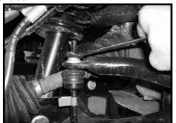
Working on the driver side, remove the nut and bolt holding the strut assembly to the lower control arm. Repeat on passenger side.
