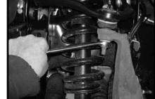
Working on the driver side, loosen but do not remove the nut from the outer tie rod. Repeat procedure on the passenger side.
