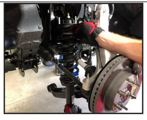
8. Using vice grip pliers, Remove the dowel pin from the strut top hat on both struts.
