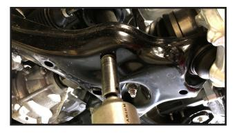
Remove the driver and passenger side lower conrol arm cam bolt nuts. Save hardware.
