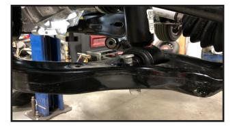
a jack, Raise lower control arms into frame mounts. Install remove the jacks. front and rear cam bolts and nuts into lower control arm mounts. Leave loose.
