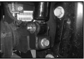
12. Working on the driver side, install the sway bar back to the sway bar end link and secure using the OE hardware. Make sure to use loctite and torque to 40 ft lbs. Repeat procedure on the passenger side.
