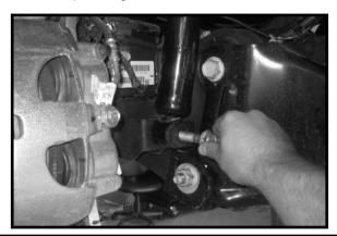
4. Working on the driver side, remove the sway bar end link from the sway bar. Save the hardware. Repeat procedure on the passenger side.
