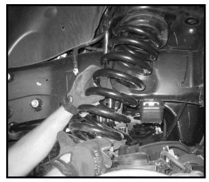
from the upper coil spring pocket and set aside. Repeat procedure on the passenger side.
