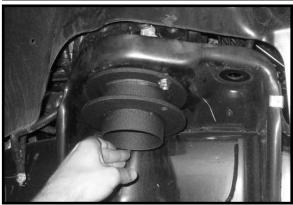
Carefully raise up on the hydraulic floor jack until the coil**front end alignment performed.** spring and isolator seat properly into the newly installed coil spring spacer. Repeat procedure on the passenger side.
