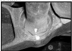
3. Working on the driver side and using a proper torsion bar removal tool. Carefully remove the torsion bar bolt and block. Set the torsion bar bolt and block aside. Remove the stock torsion bar unloading tool from the stock cross member. Special note: Tuff Country EZ-RIde Suspension requires that a proper torsion bar unloading tool be used when performing this installation. If you do not have one, please contact your local GM dealer to purchase one from them.
