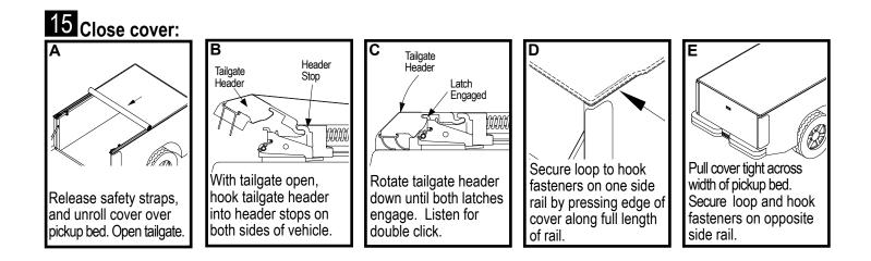
• To prevent accidental release of tailgate header, ensure header is securely latched to side rails on both sides of pickup bed before driving vehicle.
