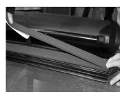
**Detail-B**: Apply the bulkhead seal to the existing seal on the underside of front header.
