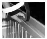
Detail-A: Apply the bulkhead seal by pealing off part of the seal's paper backing and sticking the pealed section to the bulkhead, slowly remove the paper backing as the seal is applied.
