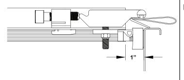
STEP 3: Side Rail Clamps: If your pickup bed does not have Utili-track channels, install three clamps on each side rail as shown in owner's Manual. If your pickup bed does have Utili-track channels, install two clamps on each side rail, locating clamps at each end of Utili-track channels.
