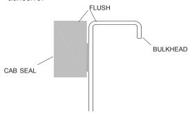
STEP 2: Side Rails: Position side rails against cab weather seals as shown below. See Owner's Manual for complete instructions.
