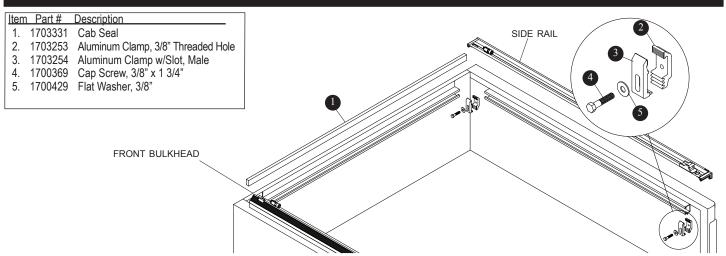
Follow these instructions to install cab weather seal and side rail clamps on your Nissan Frontier pickup. Refer to Owner's Manual for complete installation instructions.
