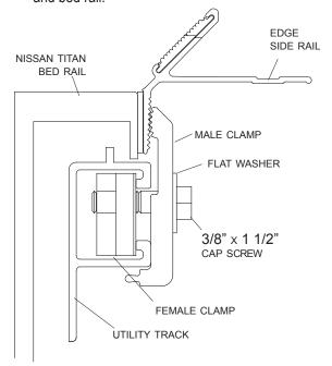
**STEP 4:** Tighten clamps securely.
