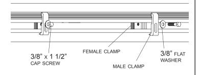
STEP 3: Install Edge side rails, wedging rails between male clamp and bed rail.
