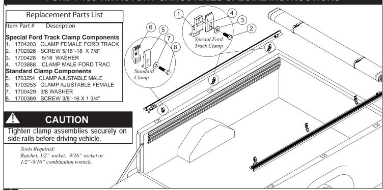
Correct clamping location: Place clamps in the locations shown below. See detail A and B for more information.
