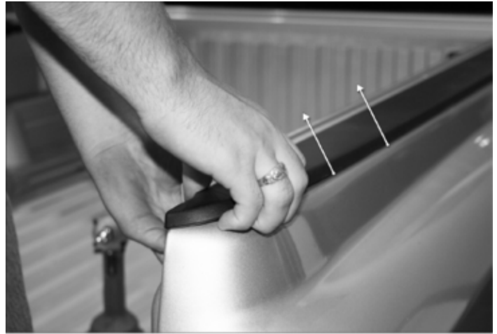
Cargo rails are held on by adhesive back tape and plastic fasteners.
