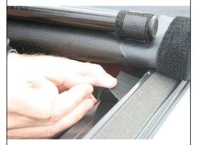
Align the edge of the 4" polyester hook strip to the edge of the side rail.
