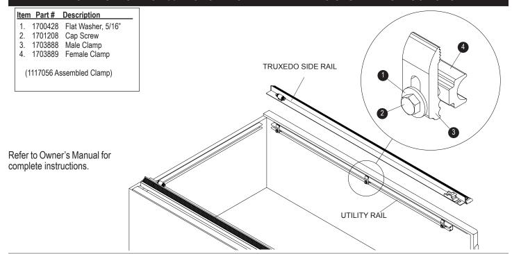
STEP 1: Insert clamp assemblies into utility rails, three on each side of pickup bed.
