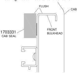
STEP 2: Position cab header over front bulkhead and cab seal as shown below. Install your Truxport cover as shown in owner's manual.
