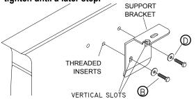
STEP 2: Align verticle slots on support bracket with threaded inserts at front of composite box. Insert screws ① through washers ① and slots in bracket. Finger tighten into composite box.
