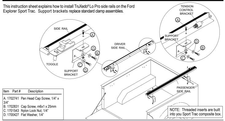
STEP 1: Align verticle slots in support bracket with threaded inserts in composite box near tailgate. Insert screws through washers • and slots in bracket. Thread the screws into composite box **DO NOT completely tighten until a later step.**
