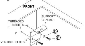
STEP 3: Fasten side rails to support brackets through holes in side rails with screws **①**, washers **①**, and nuts **②**.
