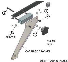
STEP 4: Replace Carriage Brackets: Slide carriage bracket assemblies into Utili-track channels. Re-install rear stop blocks and bed extender cage, following manufacturer's instructions.
