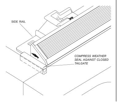
STEP 2: Back spring plungers out. Place cover assembly across pickup bed, between side rails and toolbox. If D-seal is not compressed against toolbox, move side rails toward cab.
