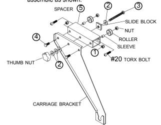
STEP 4: Replace Carriage Brackets: Slide carriage bracket assemblies into Utili-track channels at cab end of pickup bed. Slide toward tailgate. Re-install bed extender cage, following manufacturers instructions.
