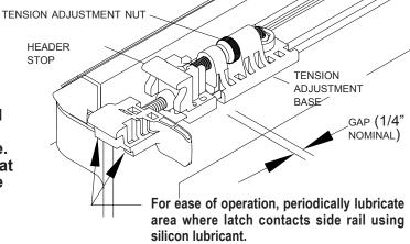
**NOTE:** Cover is designed to have optimal tension when there is a 1/4" gap between the header stop and the tension adjustment base.
