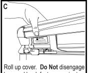
loop and hook fasteners prior to rolling up cover.
