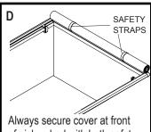
of pickup bed with both safety straps when cover is open.
