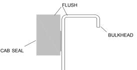
STEP 2: Side Rails: Position side rails against cab weather seal as shown below. See Owner's Manual for complete instructions.
