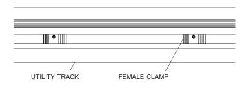
**STEP 2:** Evenly space and fasten male clamps loosely to female clamps with 3/8" x 1 1/2" cap screws.
