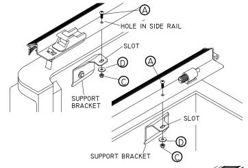
STEP 4: Adjust side rails rearward so that the curve in the side rail seals against the curve in the composite box.
