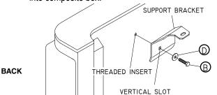
STEP 2: Align verticle slot on support bracket with threaded insert at front of composite box. Insert screw through washer and slot in bracket. Finger tighten into composite box.
