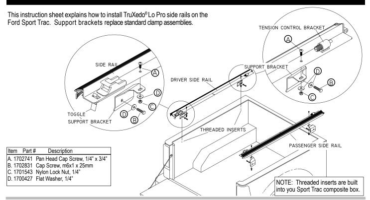
STEP 1: Align verticle slot in support bracket with threaded insert in composite box near tailgate. Insert screw ① through washer ② and slot in bracket. Finger tighten into composite box.
