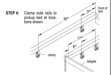
STEP 5: Align side rails 1/2" from tailgate, flush with bed rail and level with each other. Tighten clamp assemblies (see Owner's Manual).
