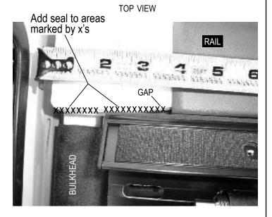
STEP 2: Cut another piece of seal and affix it to area marked by x's in the photo below.
