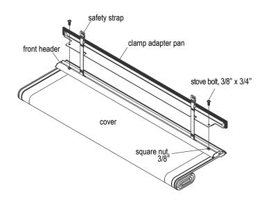
STEP 7: Front header: Back spring plunger out. Set cover assembly across cab end of side rails. Insert screws in front header through slots in side rails. Secure with plastic washers and lock nuts, but do not over tighten. Header must be free to slide.
