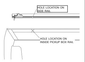
STEP 2: Make sure hole locations are about 5/8" down from top edge of pickup box. Drill 13/64" holes at marked locations.
