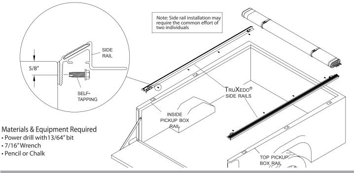
STEP 1: TruXedo<sup>®</sup> Lo Profile side rails have four prepunched mounting holes. Hold side rails against front of box, keeping offset portion of rail flush with top rail of box. Chalk mark locations of four holes on inside of pickup box, using mounting holes as guides.
