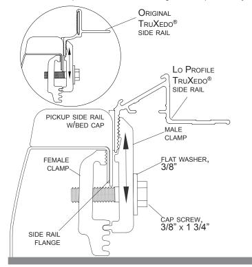
STEP 3: Attach two clamp assemblies at rear of side rail in recess of pickup box. Side rail is notched to fit on top of pickup box post.
