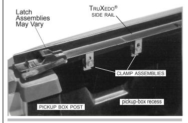
STEP 4: Mount side rail at tailgate end above bed cap as shown. Rear header seal functions best when tailgate is closed and cover is latched on top of tailgate.
