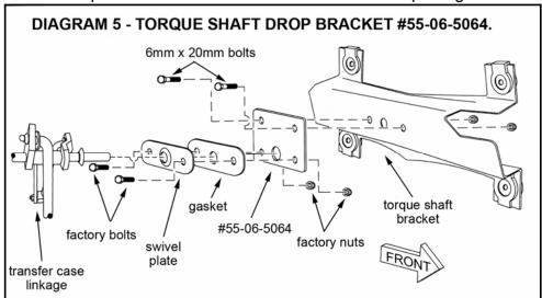
using the supplied 6mm x 20mm allen head bolts and nuts (18).
