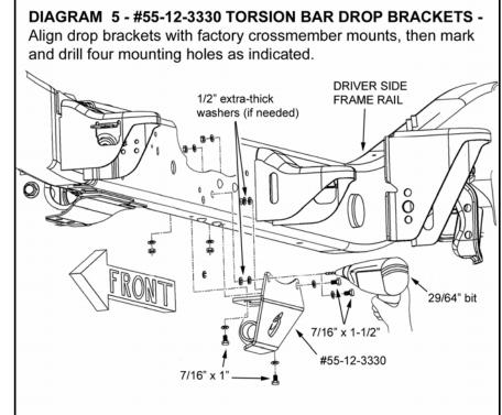
Due to variations in frame width, it may be necessary to space the drop brackets out slightly from the sides of the frame with the supplied extra-thick flat washers (up to two per side). Clamp each bracket firmly in place, then use a center punch to mark the location of the four holes to be drilled (two in the side of the frame and two in the bottom).
