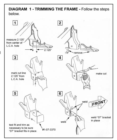
shown in Diagram 1. It may be necessary to trim the bracket in order to fit the installer's cut lines. Care should be taken to trim the piece as precisely as possible to ensure a good solid weld.
