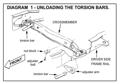
**NOTE:** Because of the extreme loads generated by the torsion bars on these vehicles, a standard two-jaw puller tool tends to bend the "lips" of the crossmember (which it uses for attachment) and may pop out of place. We have had the best results using a C-clamp type puller tool as shown. If one cannot be found locally, this tool (PN J-22517-C) is available from the Kent Moore Tool Group in Roseville, Michigan (800/345-2233 or 313/774-9500).
