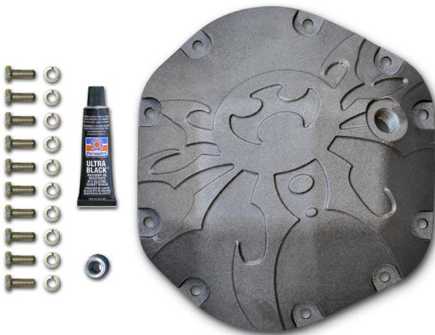
Poison Spyder Customs' Bombshell differential covers are designed to protect your differential's internals from damage due to menacing trail obstacles. Bombshells prevent cover peel back and fluid loss from broken seals. The design of the Bombshell also protects the bolt heads from trail damage while acting as a ramp, or skid, to help ease you over obstacles.
