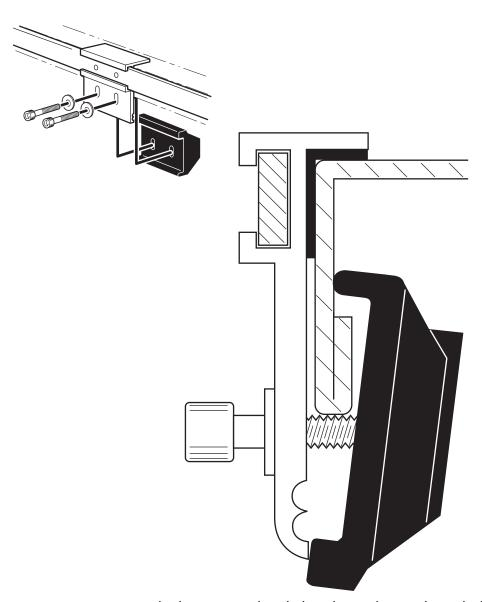
Attach clamp to each side bracket with two clamp bolts.
