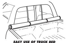
Tarp may be rolled up and secured with Velcro® for bulk hauling
