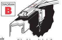
Side rail clamped to bed with bow attached.
