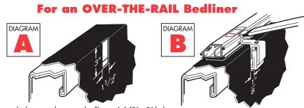
For each clamp mark on your bedliner a 1-1/2" x 3" hole as shown above. Remove clamp. Cut holes in bedliner. Reinsert side rail clamp. Return to step 6.
