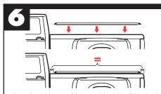
Place the rail assembly over the side of the truck box. Center rails evenly between cab and tailgate. (NOTE: Some applications have hard rubber risers (square rubber pad.) A riser must go toward tailgate. Some applications will have a riser at both ends, (most have no riser).
