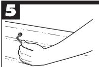
Use the included torx wrench to remove three (3) bolts on each side of truckbed wall.
