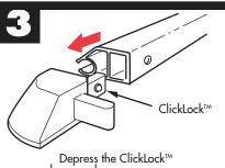
Depress the ClickLock™ release and remove one corner from cab rail.
