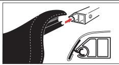
Feed tarp dowel into cab rail. (NOTE: For easiest feeding action, place tarp on a flat smooth surface, and keep dowel straight while feeding into cab rail. Caution, pavement may scuff tarp.)
