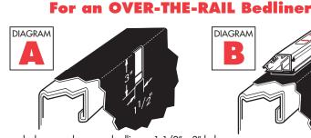
For each clamp mark on your bedliner a 1-1/2" x 3" hole as shown above. Remove clamp. Cut holes in bedliner. Reinsert side rail clamp. Return to step 6.
