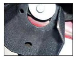
**4.** Once all the nuts have been loosely threaded and the Armor is attached to the vehicle, begin tightening the nuts to 40-ft/lbs. Repeat for each mounting location.
