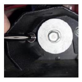
5. Once all the nuts have been tightened, tighten the center bolt of the body mount to 80-ft/lbs. Repeat for
