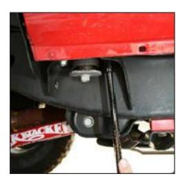
**3.** Supporting the RRC Side Armor from underneath, lift the Armor into place and slide it between the large washer and the body mount, taking care to align the holes in the Armor mount with the two body mount studs. Apply several drops of thread locker to the studs. Thread the two nuts onto the studs loosely. Repeat for each body mount location.
