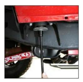
**2.** Once the center bolts are removed, remove the remaining two (2)16mm nuts located on either side of the bolt. Do this for each of the four (4) body mounts.
