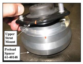
19. Torque the upper strut mounting plate retaining nut to 20 ft./lbs.
